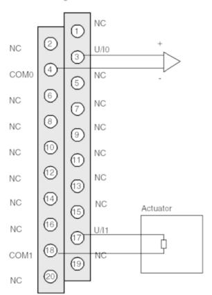
U/Ix + pole input for channel x COMx - pole input for channel x Channel 0 Voltage actuator Channel 1 Current actuator
