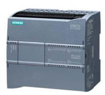
\*\*\*Spare part\*\*\* SIMATIC S7-1200, CPU 1214C, compact CPU, AC/DC/relay, onboard I/O: 14 DI 24 V DC; 10 DO relay 2 A; 2 AI 0-10 V DC, Power supply: AC 85-264 V AC at 47-63 Hz, Program/data memory 50 KB
