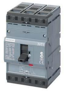
CIRCUIT BREAKER 3VT1 STANDARD BREAKING CAPACITY ICU=25KA, 415V AC 3-POLE, SYSTEM PROTECTION OVERCURRENT RELEASE TM, LI IN= 100A RATED CURRENT IR= 80... 100A OVERLOAD PROT. II= 500... 1000A, SHORT-CIRCUIT PROTECTION WITHOUT AUXILIARY RELEASE WITHOUT AUXILIARY/ALARM SWITCH
