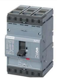
CIRCUIT BREAKER 3VT1 STANDARD BREAKING CAPACITY ICU=25KA, 415V AC 3-POLE, SYSTEM PROTECTION ELECTRONIC TRIP UNIT TM, LI IN=63A RATED CURRENT IR=50... 63A OVERLOAD PROT. II=315... 630A, SHORT-CIRCUIT PROTECTION W/O AUXILIARY TRIP UNIT W/O AUXILIARY/ALARM SWITCH WITHOUT AUXILIARY RELEASE WITHOUT AUXILIARY/ALARM SWITCH
