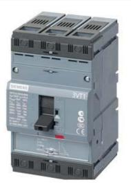
CIRCUIT BREAKER 3VT1 STANDARD BREAKING CAPACITY ICU=25KA, 415V AC 3-POLE, SYSTEM PROTECTION ELECTRONIC TRIP UNIT TM, LI IN= 40A RATED CURRENT IR= 32... 40A OVERLOAD PROT. II= 200... 400A, SHORT-CIRCUIT PROTECTION W/O AUXILIARY TRIP UNIT W/O AUXILIARY/ALARM SWITCH WITHOUT AUXILIARY RELEASE WITHOUT AUXILIARY/ALARM SWITCH
