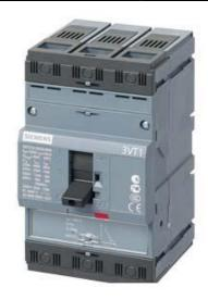
CIRCUIT BREAKER 3VT1 STANDARD BREAKING CAPACITY ICU=25KA, 415V AC 3-POLE, SYSTEM PROTECTION ELECTRONIC TRIP UNIT TM, LI IN= 20A RATED CURRENT IR= 16... 20A OVERLOAD PROT. II= 200... 300A, SHORT-CIRCUIT PROTECTION W/O AUXILIARY TRIP UNIT W/O AUXILIARY/ALARM SWITCH WITHOUT AUXILIARY RELEASE WITHOUT AUXILIARY/ALARM SWITCH
