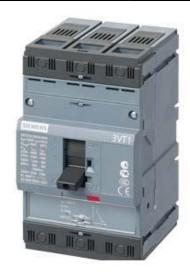
CIRCUIT BREAKER 3VT1 STANDARD BREAKING CAPACITY ICU=25KA, 415V AC 3-POLE, SYSTEM PROTECTION ELECTRONIC TRIP UNIT TM, LI IN= 16A RATED CURRENT IR= 12.5... 16A OVERLOAD PROT. II= 160... 240A, SHORT-CIRCUIT PROTECTION W/O AUXILIARY TRIP UNIT W/O AUXILIARY/ALARM SWITCH WITHOUT AUXILIARY RELEASE WITHOUT AUXILIARY/ALARM SWITCH
