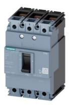
circuit breaker 3VM1 IEC frame 160 breaking capacity class N Icu=25kA @ 415V 3-pole, line protection TM210, FTFM, In=80A overload protection Ir=80A, not adjustable short-circuit protection Ii=10 x In nut keeper kit
