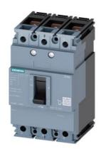
circuit breaker 3VM1 IEC frame 160 breaking capacity class N Icu=25kA @ 415V 3-pole, line protection TM210, FTFM, In=40A overload protection Ir=40A, not adjustable short-circuit protection Ii=10 x In nut keeper kit
