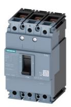
circuit breaker 3VM1 IEC frame 160 breaking capacity class N Icu=25kA @ 415V 3-pole, line protection TM210, FTFM, In=25A overload protection Ir=25A, not adjustable short-circuit protection Ii=12.8 x In nut keeper kit
