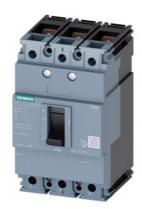
circuit breaker 3VM1 IEC frame 160 breaking capacity class N Icu=25kA @ 415V 3-pole, line protection TM210, FTFM, In=20A overload protection Ir=20A, not adjustable short-circuit protection Ii=16 x In nut keeper kit
