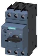
Circuit breaker 22 A A-release 17...22 A, N-release 286 A, for motor protection, class 10, screw connection, standard switching capacity,
