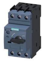
Circuit breaker 20 A A-release 13...20 A, N-release 260 A, for motor protection, class 10, screw connection, standard switching capacity
