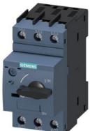
Circuit breaker 12.5 A A-release 9...12.5 A, N-release 156 A, for motor protection, class 10, screw connection, standard switching capacity
