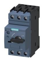
Circuit breaker 10 A A-release 7...10 A, N-release 130 A, for motor protection, class 10, screw connection, standard switching capacity  $\frac{1}{2}$
