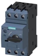
Circuit breaker 8 A A-release 5.5...8 A, N-release 104 A, for motor protection, class 10, screw connection, standard switching capacity
