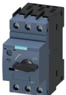
Circuit breaker 5 A A-release 3.5...5 A, N-release 65 A, for motor protection, class 10, screw connection, standard switching capacity
