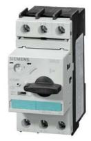
Circuit breaker size S0 For transformer protection A-release 4.5...6.3 A Short-circuit release 130 A Screw terminal Standard switching capacity !!! Phased-out product !!! Successor is SIRIUS 3RV2 Preferred successor type is >>3RV2411-1GA10<<
