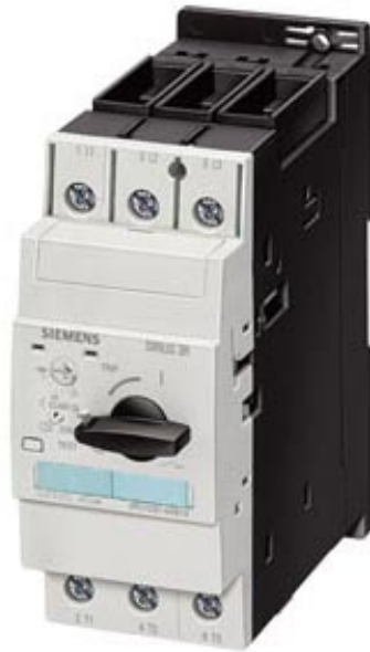
CIRCUIT-BREAKER 36...45 A, N-RELEASE 585 A, SIZE S2, MOTOR PROTECTION CLASS 10 SCREW CONNECTION STANDARD BREAKING CAPACITY
