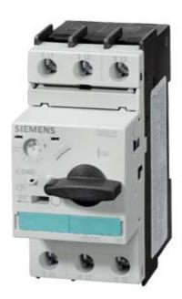
CIRCUIT-BREAKER SIZE S0, FOR MOTOR PROTECTION, CLASS 10, A-REL.0.45...0.63A,N-REL.8.2A SCREW TERMINAL, STANDARD SWITCHING CAPACITY
