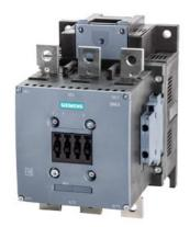
Contactor 220...240 V AC/DC AC3 110 kW 400 V AC (50...60 Hz) / DC operation auxiliary contacts 2 NO + 2 NC 3-pole, size S10 bar connections conventional operating mechan. screw terminal
