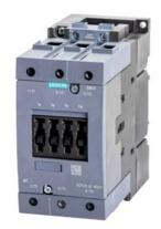
Contactor AC 220 V 50/60 HZ AC3 30 kW 400 V 3-pole, size S3 screw terminal
