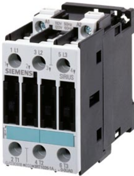
CONTACTOR, AC-3 11 KW/400 V, AC 110V 50/60HZ, 3-POLE, SIZE S0, SCREW CONNECTION
