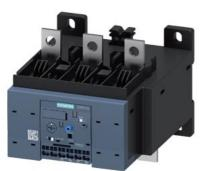
Overload relay 50...200 A for motor protection Size S6, Class 10E Contactor mounting/stand-alone installation Main circuit: busbar connection Auxiliary circuit: Spring-type terminal Manual-Automatic-Reset
